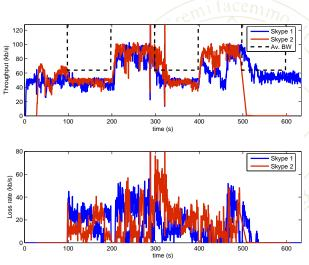
**Set-up**: Square-wave available bandwidth  $(A_{Max}=144 \text{ kb/s}, A_{min}=64 \text{ kb/s}, T = 200 s)$ . The second Skype calls is placed after 25 s.
