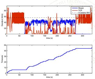
**Set-up**: Constant link capacity of 56 kb/s. Skype call starts 70 s later than the TCP flow.
