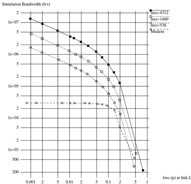
Figure 15: Effect of loss rate at link  $L$ . While modem users (with a 1000 byte MSS) do not notice loss on link  $L$  until it is quite high, R&E users suffer severe performance degradation, particularly when using a small  $MSS$ .
