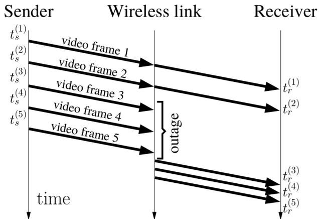
**Figure 4: Effect of a wireless channel outage on the arrival time of groups of packets (in this example a video frames fits in one group of packets)**
