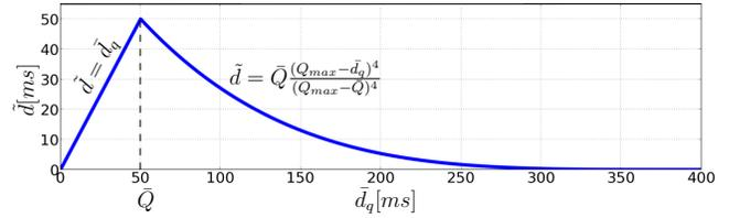
Fig. 2: Non-linear function mapping  $\bar{d}_q$  to  $\tilde{d}$
