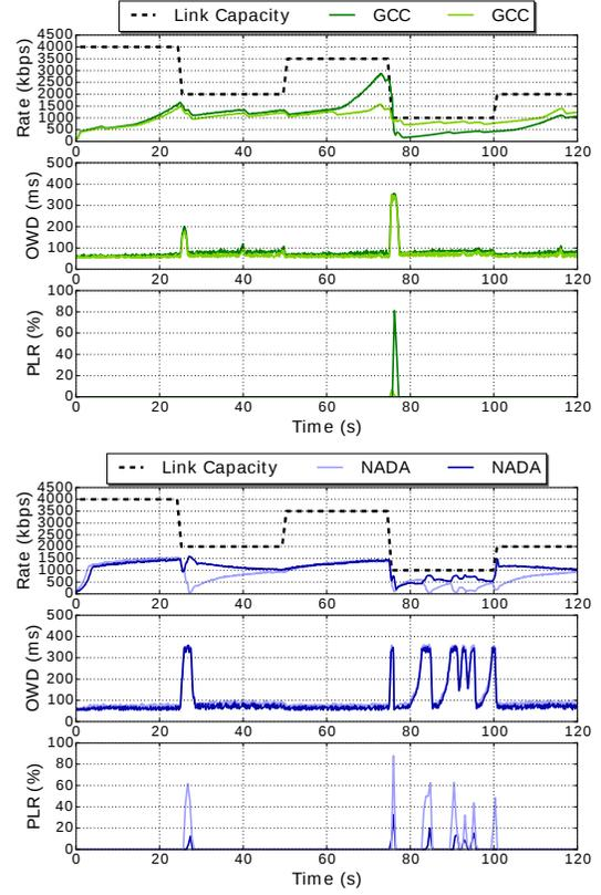
Fig. 8: Sending Rate, one-way delay (OWD) and packet loss ratio (PLR) dynamics in the case of two GCC or two NADA flows over a link with variable capacity
