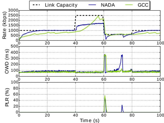
Fig. 6: Sending Rate, one-way delay (OWD) and packet loss ratio (PLR) dynamics in the case of a single GCC or NADA flow with variable link capacity
