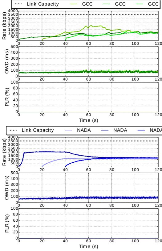
Fig. 7: Sending Rate, one-way delay (OWD) and packet loss ratio (PLR) dynamics in the case of three concurrent GCC or NADA flows over a 3.5Mbps link
