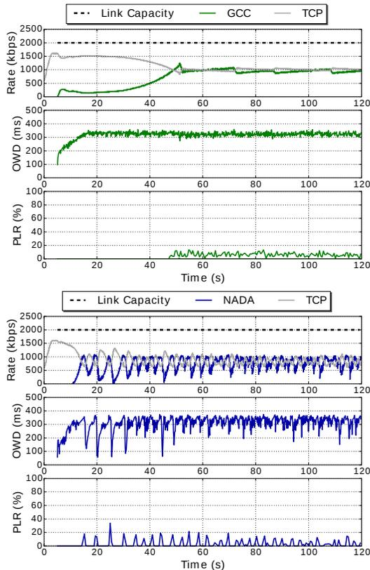
Fig. 9: The case of one GCC or NADA flow sharing a 2Mbps link with 1 TCP flow
