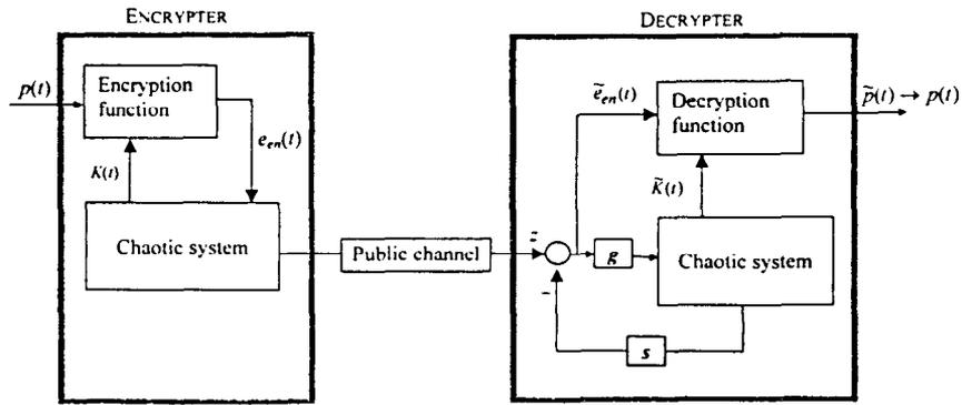
Fig. 1 A block diagram illustrating the proposed secure communications scheme.
