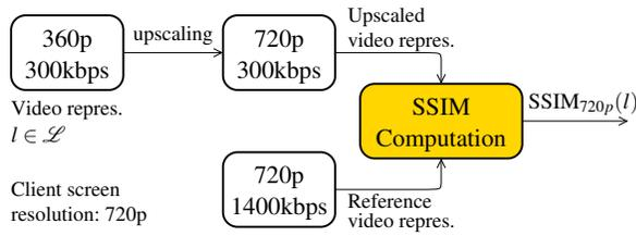
**Figure 4: SSIM computation for the video representation  $l$  (300kbps, 360p): the video representation is first upscaled to the client resolution 720p and then compared to the corresponding reference video representation (1400kbps, 720p).**
