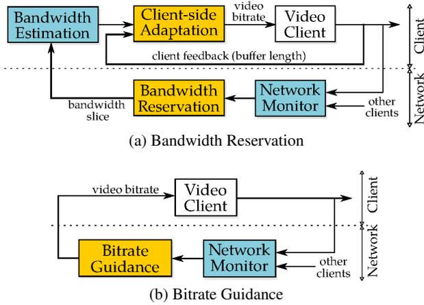
**Figure 1: Network-assisted approaches for adaptive video streaming**
