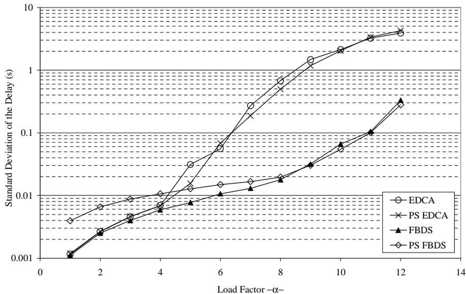
Fig. 4. Standard deviation of one-way delays of MPEG4 flows as a function of the load factor  $\alpha$ .
