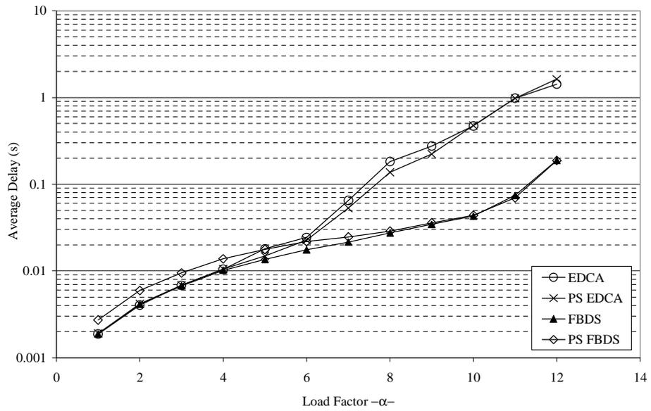
Fig. 8. Average one-way delays of H.263 flows as a function of the load factor  $\alpha$ .
