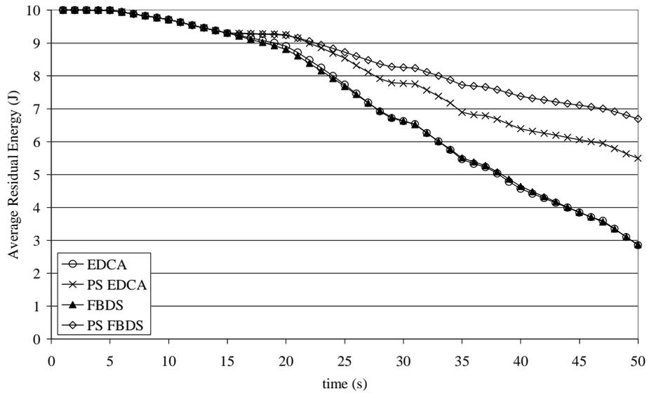
Fig. 6. Average Residual Energy for a node hosting a MPEG-4 flow when  $\alpha = 6$ .
