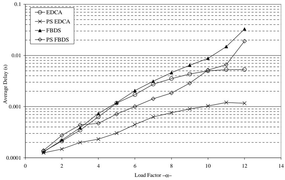
Fig. 13. Average one-way delays of G.729 flows as a function of the load factor  $\alpha$ .
