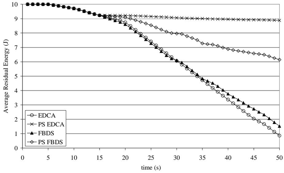
Fig. 15. Average Residual Energy for a node hosting a G.729 flow when  $\alpha = 9$ .
