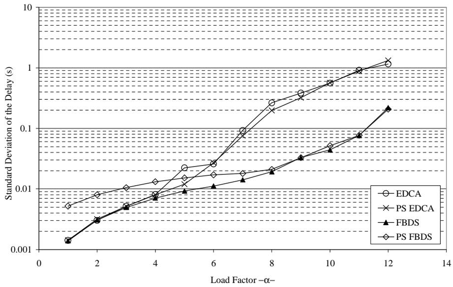
Fig. 9. Standard deviation of one-way delays of H.263 flows as a function of the load factor  $\alpha$ .
