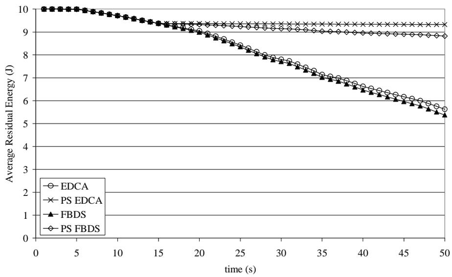
Fig. 17. Average Residual Energy for a node hosting a G.729 flow when  $\alpha = 3$ .
