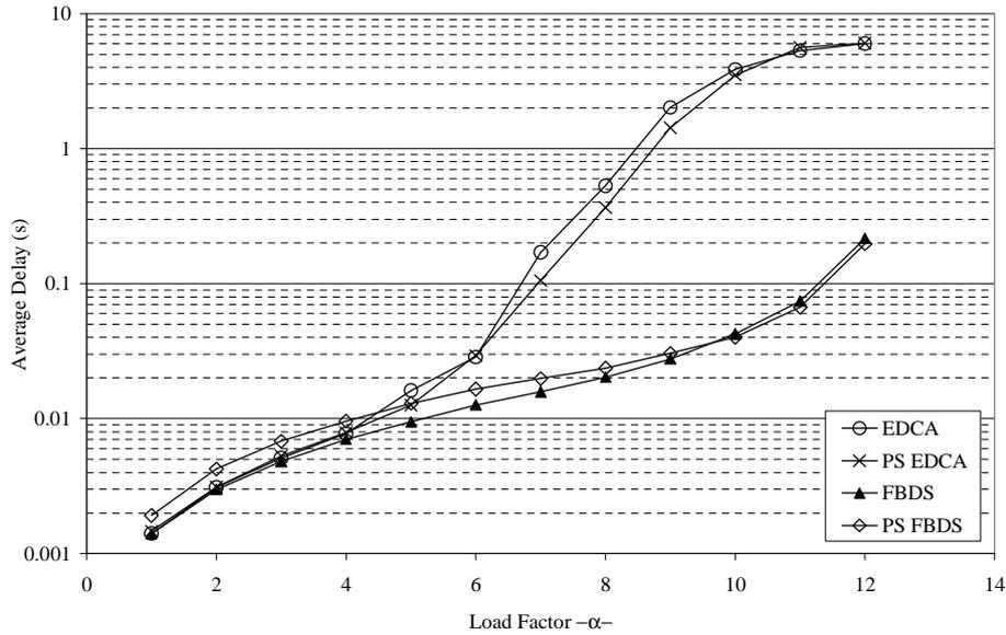
Fig. 3. Average one-way delays of MPEG4 flows as a function of the load factor  $\alpha$ .
