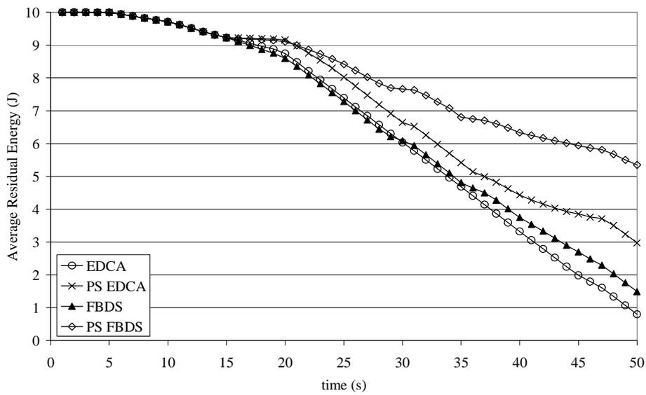
Fig. 10. Average Residual Energy for a node hosting a H.263 flow when  $\alpha = 9$ .
