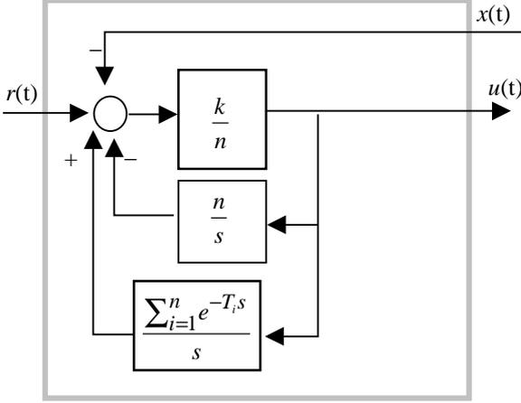
**Fig. 4:** Block diagram of the controller  $G(s)$
