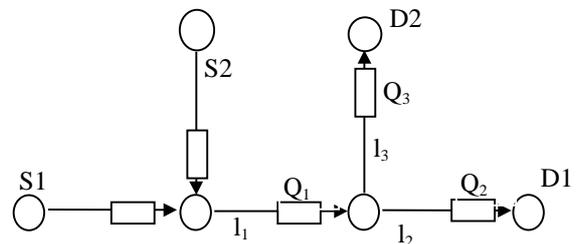
**Fig. 1:** Scheme of connections  $(S_1,D_1)$  and  $(S_2,D_2)$  sharing link  $l_1$  and queue  $Q_1$ .
