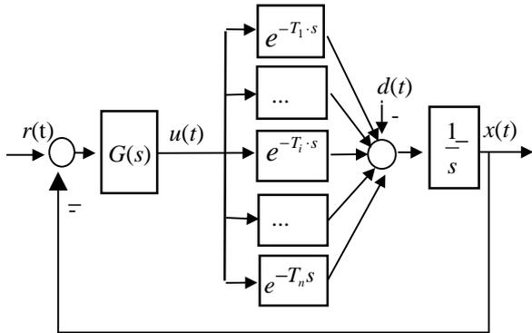
**Fig. 2:** Block diagram of  $n$  VC connections sharing a common FIFO queue
