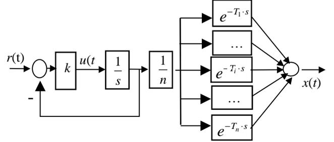
**Fig. 3:** Block diagram of the desired input-output dynamic
