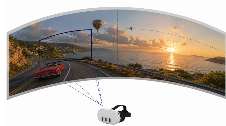
Figure 1. Viewport in tile-based 360° video streaming using ERP projection with 3 \times 4 tile grid.
